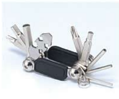
Model YC-289 Mini folding tool (nomenclon with stainless steel) 2/3/4/5/6mm hex key wrench, +/- screwdriver, T25 wrench, 3.2/3.3/3.5 and Mavic spoke wrench. PE: 100pcs/10kgs, 11kgs/0.4'
