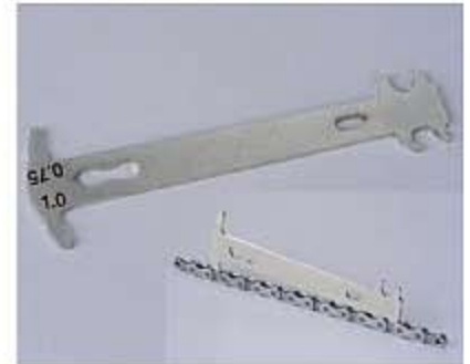
Model YC-503 Chain Wear Indicator A worn chain shifts poorly and wears sprockets at an accelerated rate. 75% and 1% wear, the points at which most chain manufacturers suggest replacement. Made from precision, laser cut steel.
